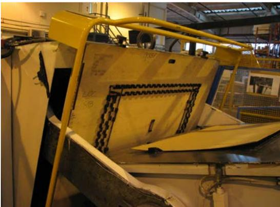
The guard is more effective on the smaller machines where it offers hand arm protection against being trapped when the platens begins to close.
