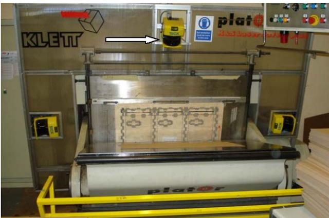
The Current EN and draft ISO Standards make reference to the provision of a laser scanner to provide front protection.
