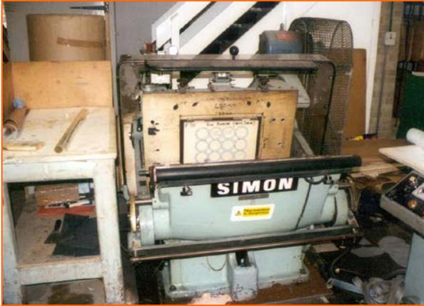
This option may be particularly suitable for smaller machines where the side tables act as both a table for storing blanks and 'processed board' and as a 'protective structure' that prevents access to the hazard zone. They are easy to produce and represent a cost effective solution.
